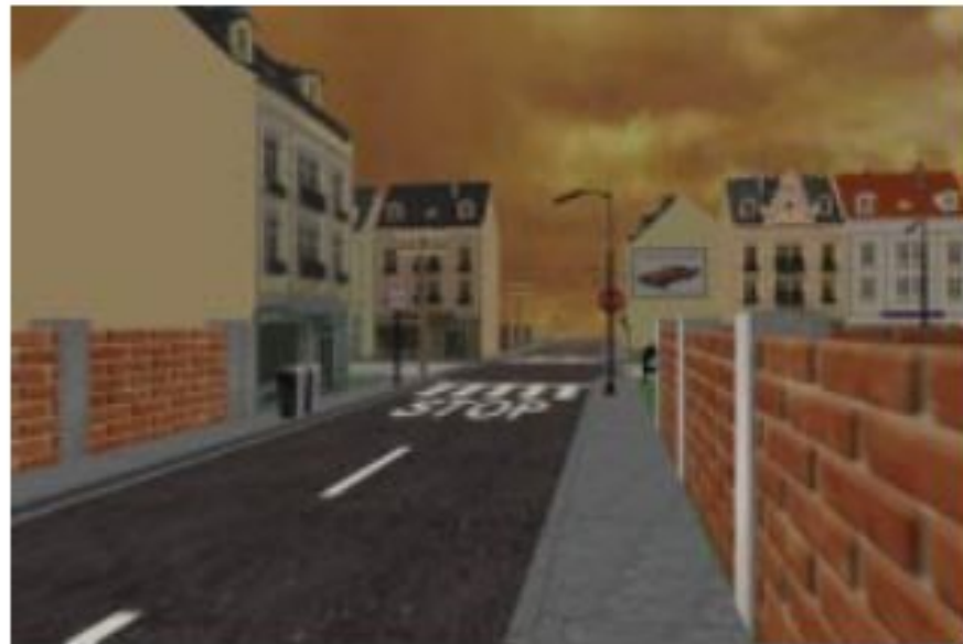
Figure 2. Same view as in Figure 1 rendered using relief texture mapping. Both scenes contain the same number of polygons. Notice the bricks standing out and the protruding domers.
